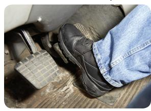
as if the brakes are pushing back at you. At times, you will feel the pedal suddenly drop. The valves in the ABS unit may make a grinding, scraping, or buzzing noise. This means your ABS is working. Continue to apply firm pressure and steer. Do not take your foot off the brake pedal.
